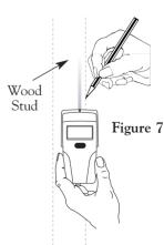
You need to locate either two studs or three studs, depending on the size of your TV. To determine whether you need two studs or three, simply refer to how you positioned the wall plate extensions in the previous step. If you extended the wall plate into or past the third expansion slot, you need to mount to three studs. If you did not extend your bracket at all, or extended it less than three slots, you can mount into only two studs.
